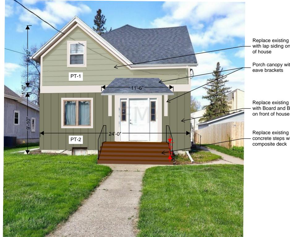
Replace existing siding with lap siding on front
