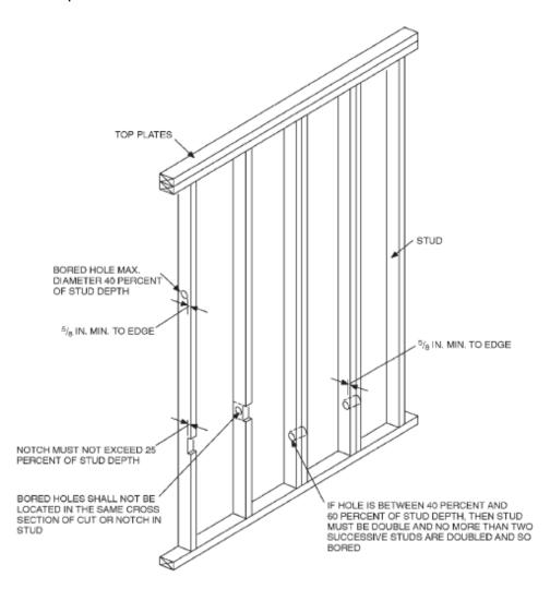
**R602.5 Interior nonbearing walls.** Interior nonbearing walls shall be permitted to be constructed with 2-inch-by-3-inch (51 mm by 76 mm) studs spaced 24 inches (610 mm) on center or, when not part of a *braced wall line*, 2-inch-by-4-inch (51 mm by 102 mm) flat studs spaced at 16 inches (406 mm) on center. Interior nonbearing walls shall be capped with at least a single top plate. Interior nonbearing walls shall be fireblocked in accordance with Section R602.8.
