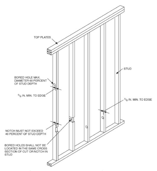
**R602.6 Drilling and notching–studs.** Drilling and notching of studs shall be in accordance with the following:
