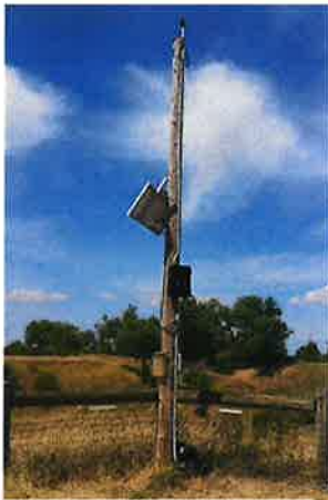
Permanent Noise Monitor with Remote Website Access
