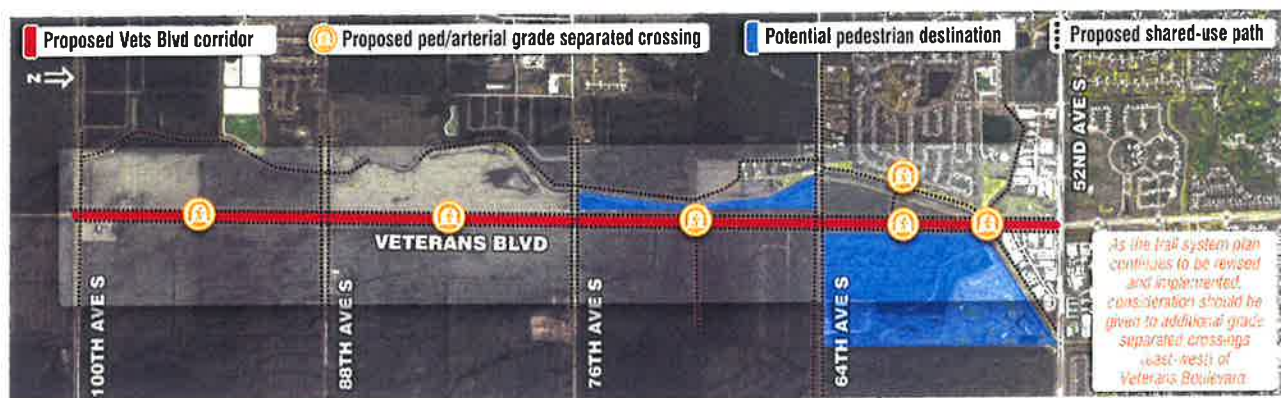
Figure 23, Future Bicycle and Pedestrian System Considerations
