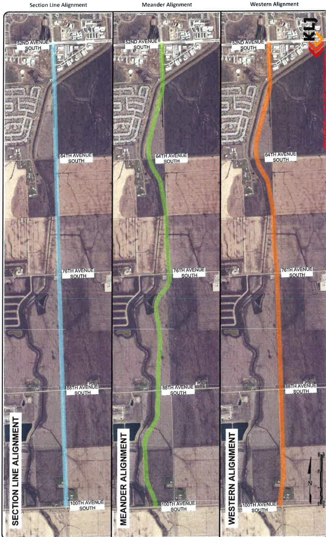
Figure 5: Veterans Boulevard Extension Corridor Alignment Alternatives
