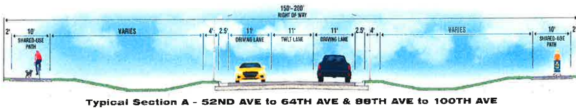
Figure 16: Typical Section A (Facing North)
