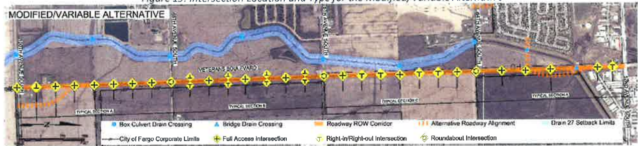
Figure 19: Intersection Location and Type for the Modified/Variable Alternative
