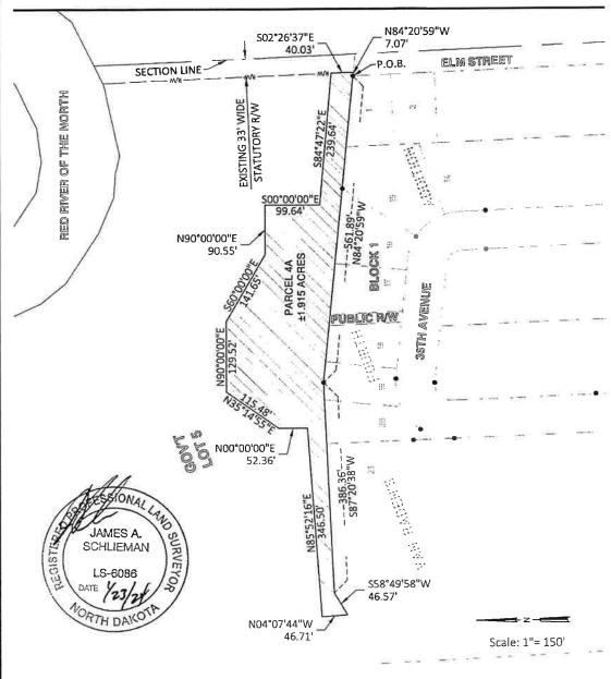
IRON MONUMENT FOUND MEASURED BEARING MEASURED DISTANCE PERMANENT EASEMENT TEMPORARY EASEMENT
