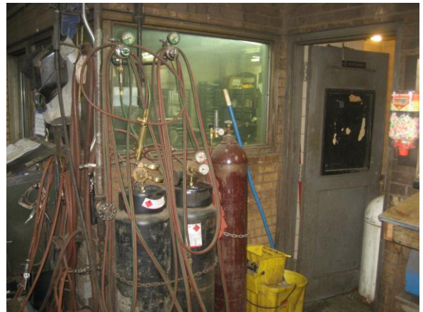
Photo #16 Acetylene and Oxygen Tanks Inside Structural Steel Fabrication Shop #2
