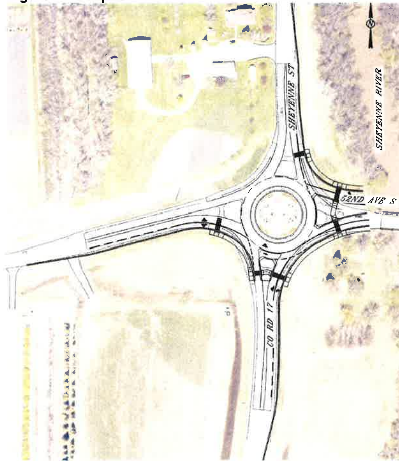
Figure 1 – Proposed 2x1 Roundabout Construction
