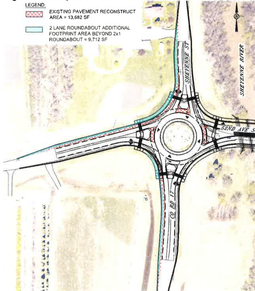
Figure 3 – Comparison of 2x1 Roundabout and Full Two-Lane Roundabout
