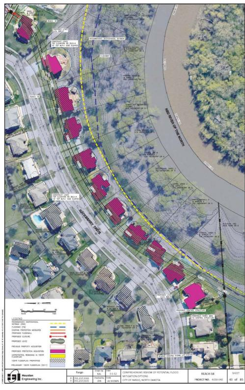
64th Ave South West of Rosewood Acquire & Deconstruct 5 Homes, 29 Levee Construction/Road Raise Levee Construction Larwood Dr. Acquire Prairie Rose Acquire & Deconstruct 35 Homes. Deconstruct 2 Homes, Levee/Floodwall **Levee Construction** Construction Belmont Park Acquire & **Deconstruct 30 Homes** Levee Construction
