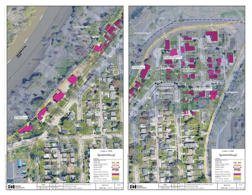
West of I-29 S Drain 27 42<sup>nd</sup> to 45<sup>th</sup> Street Acquire & Deconstruct 22 Twin-homes, Levee Construction Drain 27 40th to 44th Ave Levee/Floodwall Construction Drain 27 44th Ave to 52nd **Ave Levee Construction** 64th Ave S East of D53 Levee Construction
