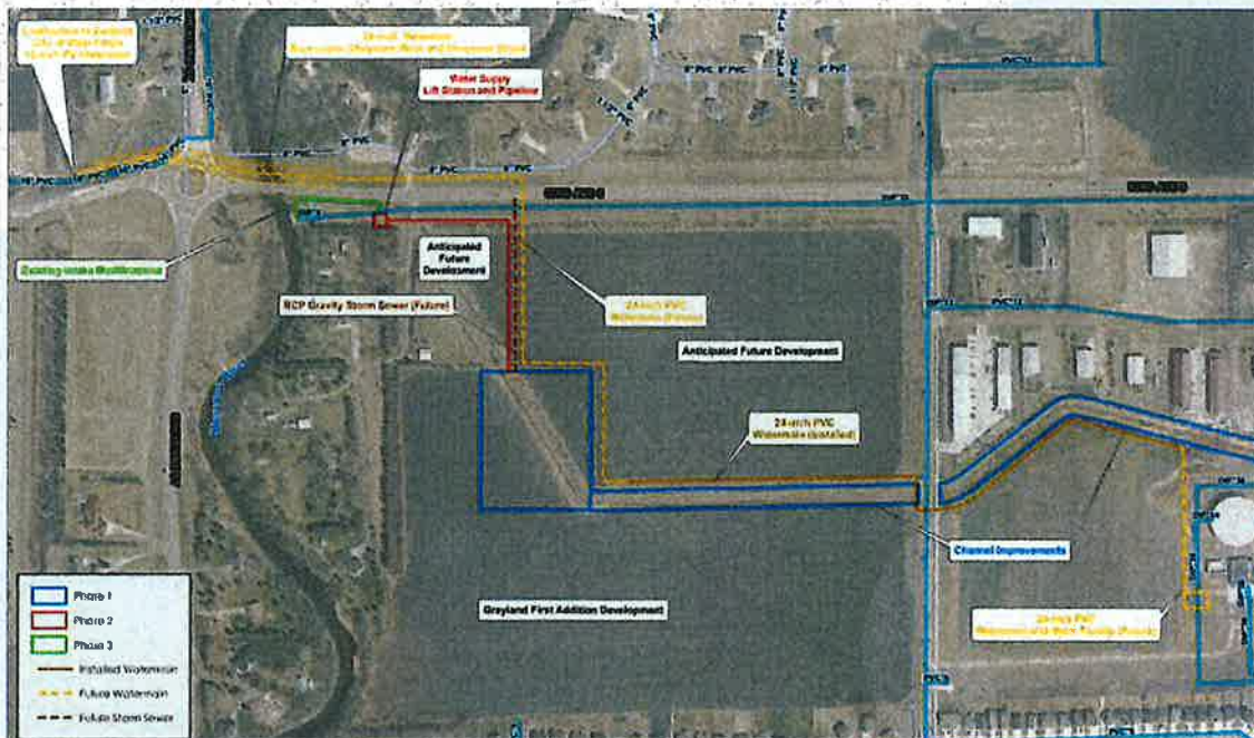
Diagram shows phases of 3 rd West Fargo Water Service Connection & Drain Improvements for Storm Water Management and Water Supply to the Water Treatment Plant.
