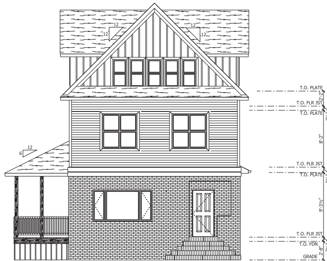
FRONT ELEVATION SCALE: 1/4" = 1'-0"
