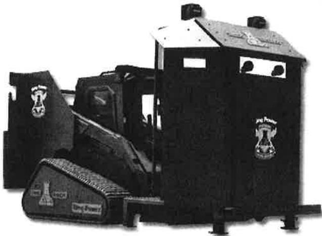
When the Armored Deployment Platform is mounted on the vehicle, the operator can raise it to 11 feet so that entry can be made on both the first and second floors, and the roofs. The platform height is also ideal for airplane assault incidents. In a vehicle take down, the platform can be slanted downward for crowd control and rescues.
