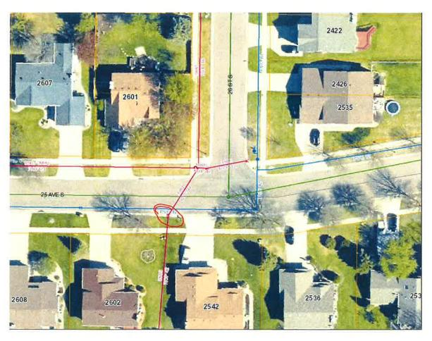
The Public Works Department discovered a large amount of gravel in the pipes and it appears to have come from a deteriorated pipe/manhole connection. There is a large void (depth in excess of four-foot probe) under the asphalt pavement and the limits of the void are unknown until the pavement is removed.
